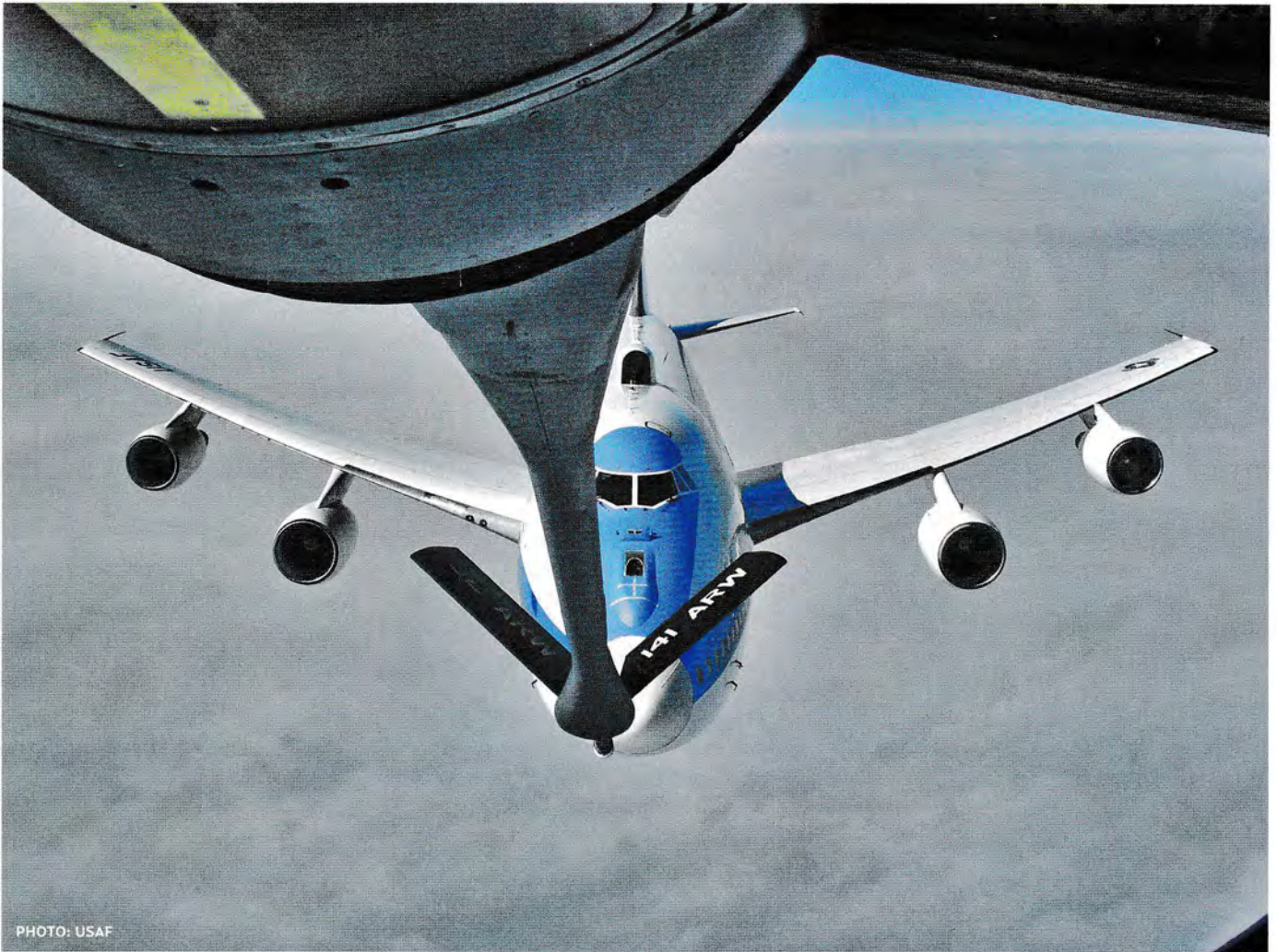
E-4B with air refueling receptacle doors open, about to be 'plugged' by a KC-135 tanker.
