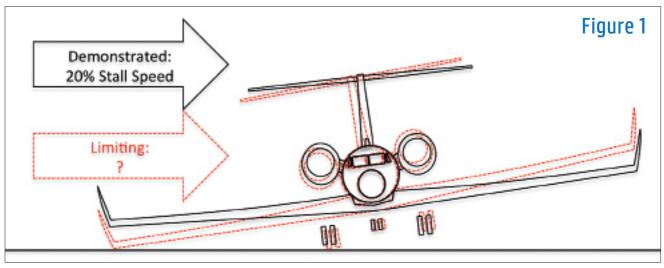
less than the point a wing-low landing scrapes a wingtip or engine pod? We can all agree that is taking things too far. But how close to limiting should the manufacturer go?
