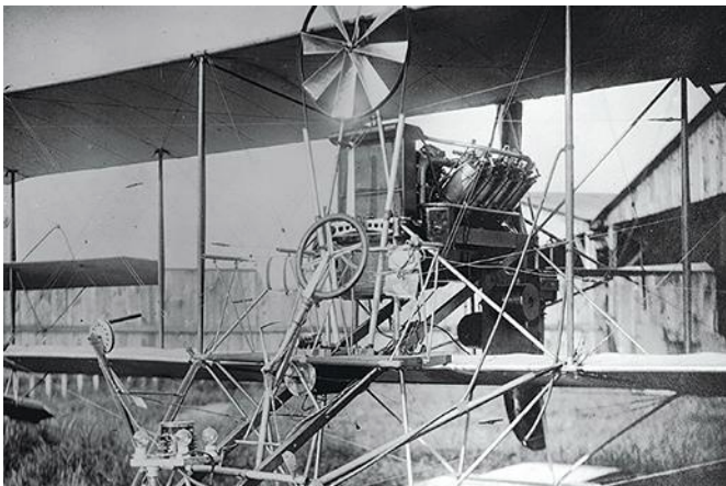
Sperry autopilot installed on a Curtiss biplane. (Glenn H. Curtiss Museum)
