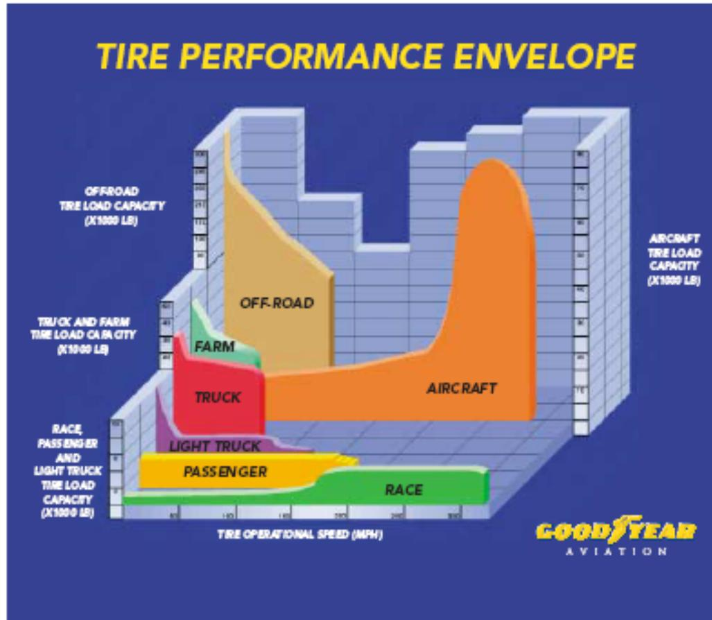
Aircraft speed and load requirements are most severe
