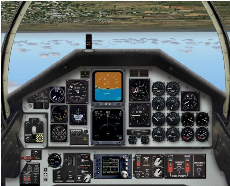
**1.2. Control and Performance Concept.** The pilot establishes an attitude and power setting that will result in the desired aircraft performance, trims the aircraft for hands-off flight, and references the performance instruments. If deviations occur, power and attitude corrections are made and the process repeats. In general, small smooth corrections coupled with an efficient
