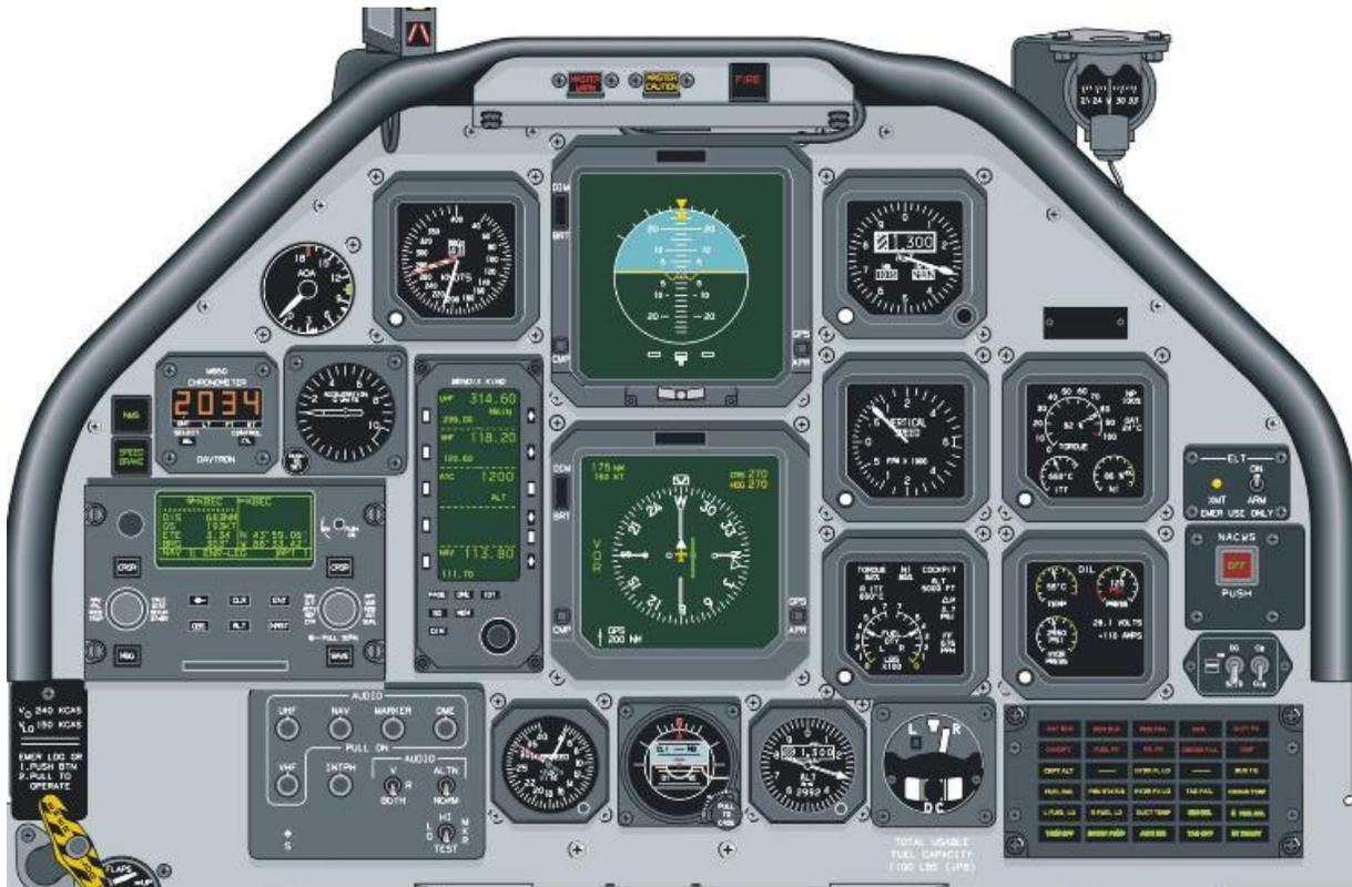
**1.3. Display of Flight Instrumentation (Figure 1 3).** Display options vary widely from aircraft to aircraft and incorporate different symbologies and terminology for similar functions. Electronic displays allow the pilot to optimize cockpit instrumentation for a particular mission by decluttering, removing, or relocating presentations. However, with very few exceptions, Air Force instrument cockpits must adhere to the following specific rules of instrumentation, equipment and setup:
