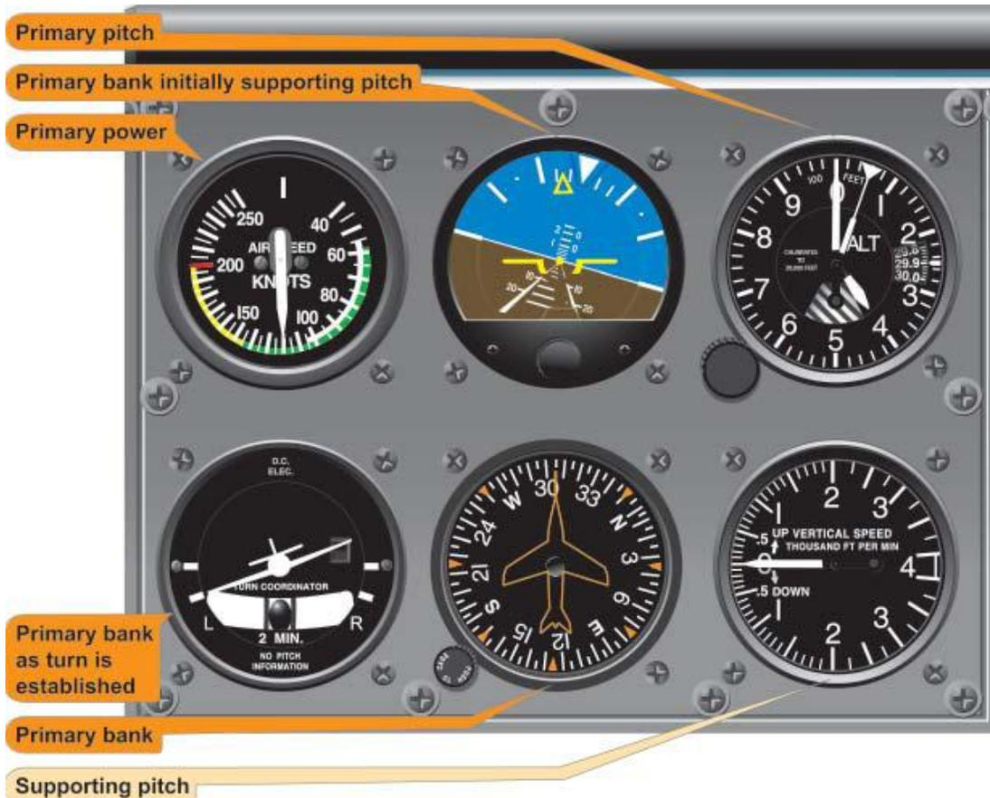
2.3.2.3. To roll out of a turn on a desired heading, calculate a lead point that is, as a guide, approximately one-third the angle of bank used in the turn. (Figure 2.4) When the lead point is reached, simply reverse the bank, pitch, trim and power inputs used to roll into the turn, smoothly and simultaneously. Once on the new heading, check for deviations from straight and level flight and apply corrections as needed.
