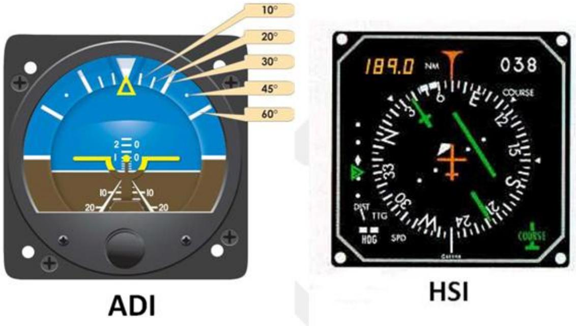
3.3.1.1.2. Command Bars. The command bars display steering information to intercept or maintain a desired flight path. To utilize the steering function, simply “fly” the ADI’s aircraft symbol by adjusting the aircraft attitude until it is snugly aligned beneath the command bars. The bars will command the proper pitch and bank to turn, intercept, and maintain a course and altitude.
