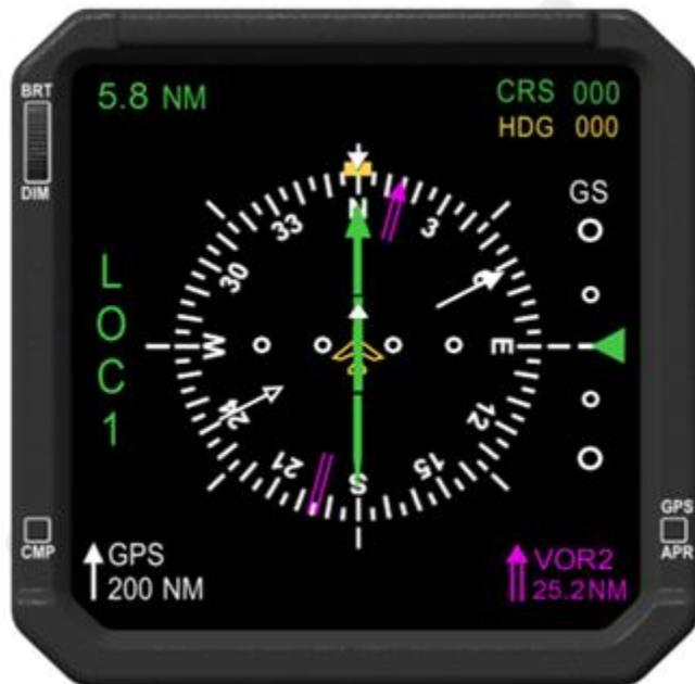
3.3.2.1. Course Selector Knob. The course selector knob on most HSI's may be used to select any course by rotating the head of the course arrow to the desired course on the compass card. Check the course selector window for the proper setting.
